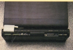
The rear of the MTX 512 showing the ribbon cable for connection to the FDX disk drives.
